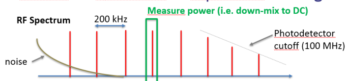
Figure 49 : (left, top) Operation principle of the supercontinuum. (left, bottom) Working principle of the detection scheme. (right) Measured supercontinuum spectrum.
