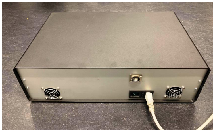
Figure 23 : Packaged LW-MIR FLAIR supercontinuum source in a 474 x 300 x 134.5mm box.
